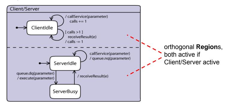
orthogonal states are "concurrent" as a single event may trigger a transition in each orthogonal region "simultaneously"
