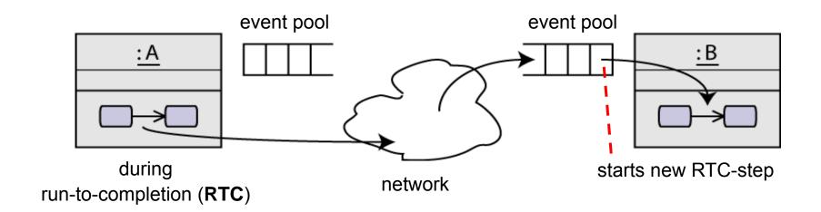
signals: asynchronous (no waiting)
