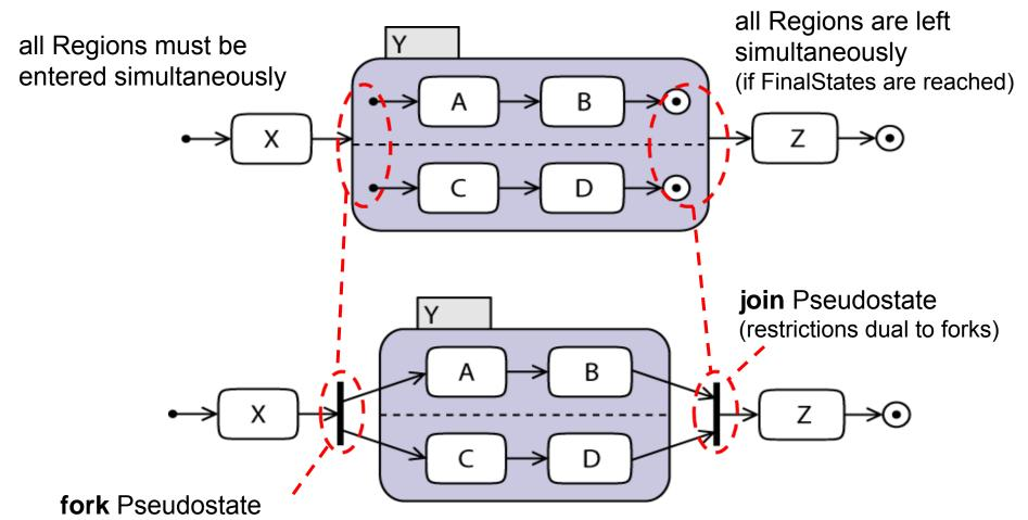
(one incoming, at least two outgoing Transitions; outgoing Transitions must target States in different Regions of an orthogonal State)
